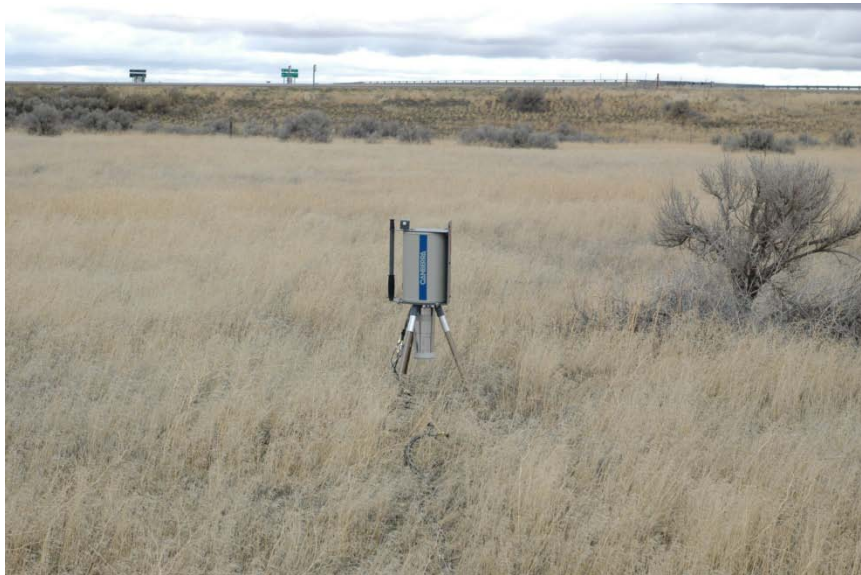
Photograph 6: HPGe Detector Mounted on a Detector Stand
