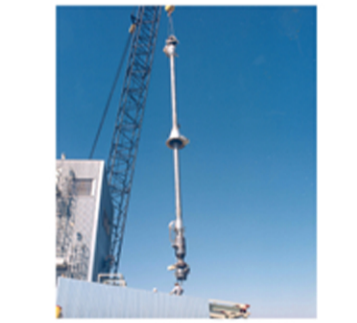
Few-Tube Test Model – Tested the concept of incorporating steam leak detection into the tube design of a sodium/steam heat exchanger.
