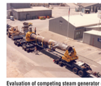
Evaluation of competing steam generator designs - The SCTI was used to test and compare competing engineering designs. The 75 megawatt steam generator on the left was designed by Atomics International while the similar sized unit on the right was designed by Babcock and Wilcox.
