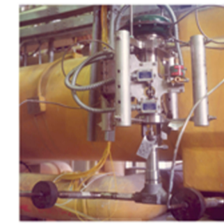
Sodium Valves – Valves to control high temperature sodium were tested with the results used to evaluate and verify a variety of designs.
