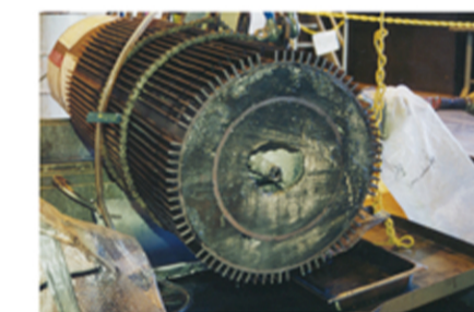
Sodium Cold Traps – High sodium purity was maintained by using this device to cool and isolate impurities. This cold trap has been cut open and solid sodium is seen within.
