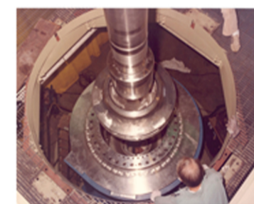
Mechanical Sodium Pumps – Research into designing efficient, high flow mechanical pumps was performed. Many pumps were developed.
