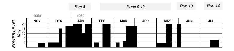
• **Run 8** Oxygen contamination observed in sodium; higher than expected temperatures observed in some channels
