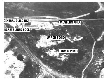
After testing, we brought equipment and piping to this site for cleaning. The first step in the cleaning process was to steam clean the equipment to remove the sodium that was easy to reach. The components were then placed in the concrete pool so they could react with water. In the final step, we placed the parts in the ponds to gradually remove any
