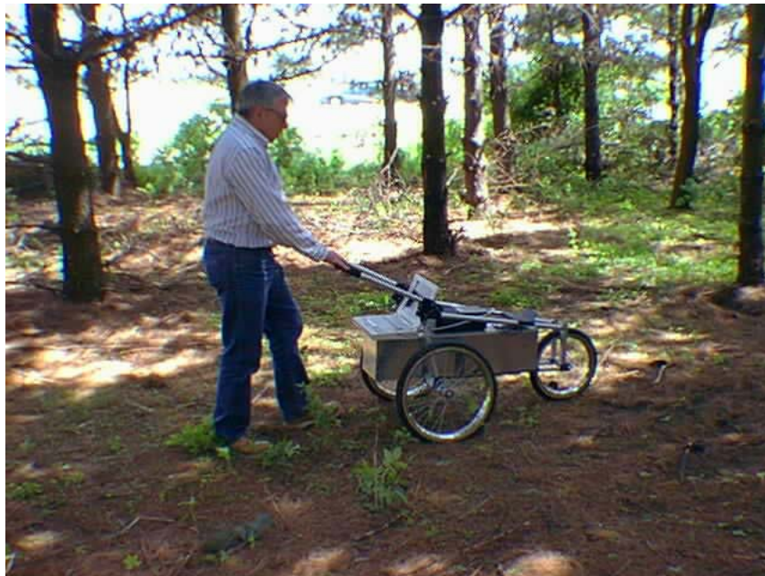
Photograph 4: Cart with 4-inch by 4-inch by 16-inch Sodium Iodide Detector
