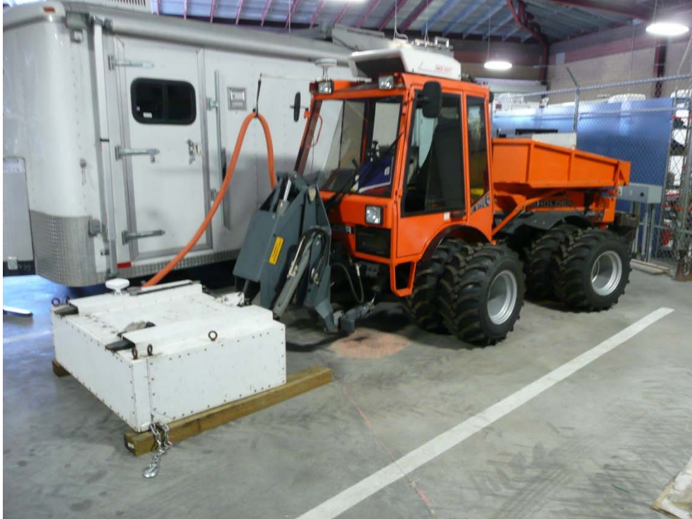
Photograph 1: EPA ERGS detection system mounted on a tractor
