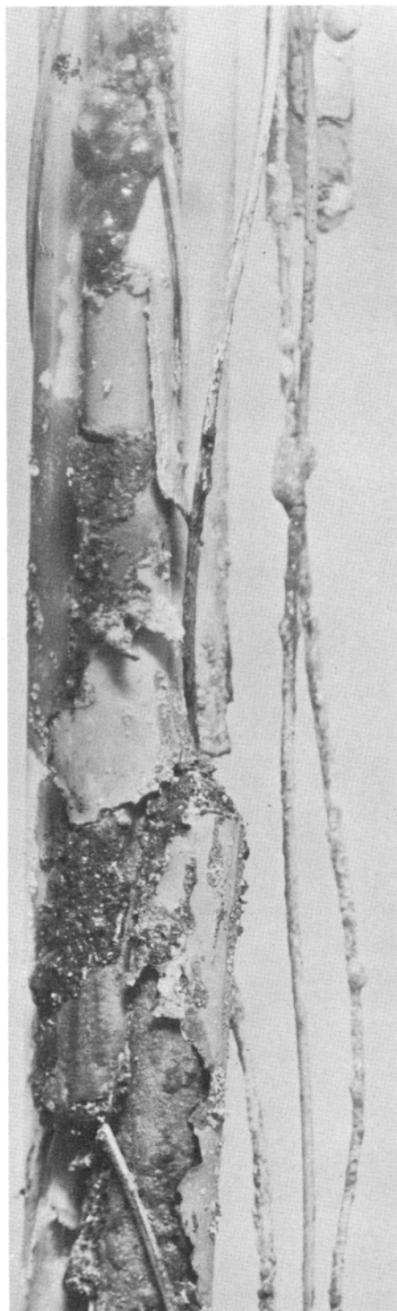
Figure IV-A-7. Midsection of Damaged Element in Channel 55
