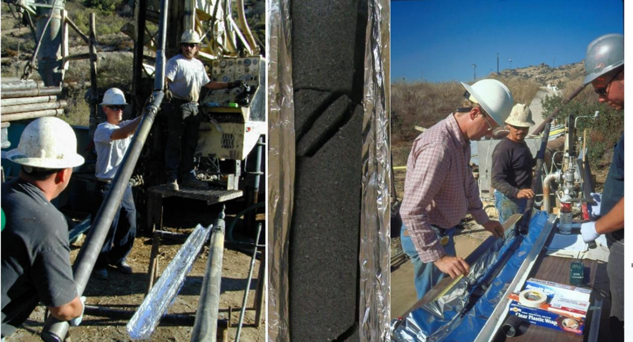
Retrieval of core in 5 fool lengths is followed by photographing, visual inspection and recording of hydrogeologic properties including; fractures, lithology, mineralogy etc.
